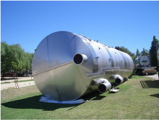
(a) One of the triple stacked stainless steel tanks to replace the old concrete tanks in Store D.
