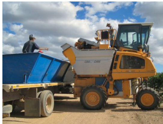
(b) A harvester as seen from the side, about to load the picked grapes into a transportation vehicle.
