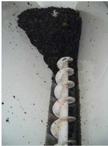
(c) Grapes being loaded into the tipping bin and moved into the crusher/destemmer using the worm.
