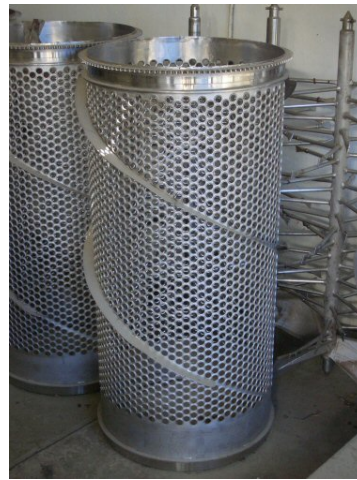
(d) The central component of the mechanical destemming machine and the multi-paddle instrument on its right.
