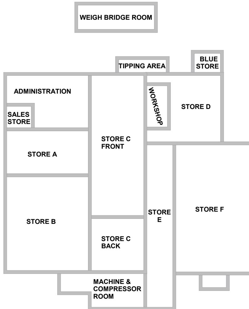
Figure 4.3: A floor plan of the cellar layout at Wamakersvallei, showing its seven functional areas [135].
