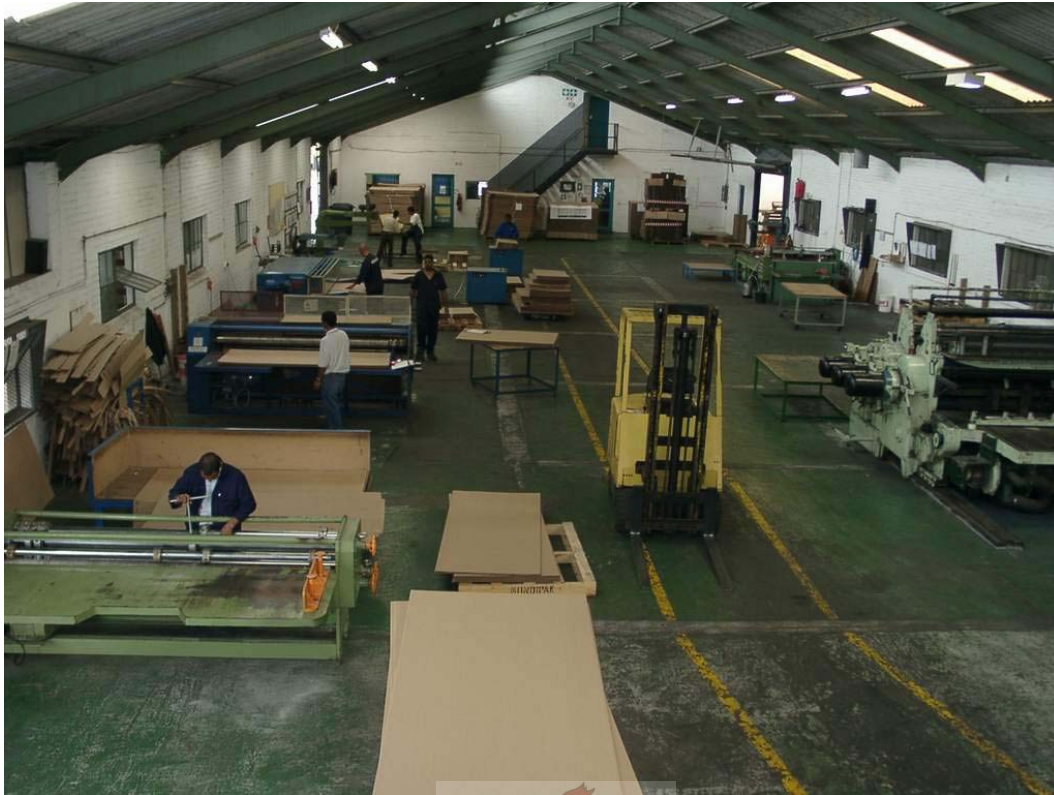
Figure 3.6: The production area, where the manufacturing of boxes takes place. The machinery is organised in two production lines, on either side of the central aisle. The production line on the left of the photo is used for small order batches and the line on the right is used for large order batches.
